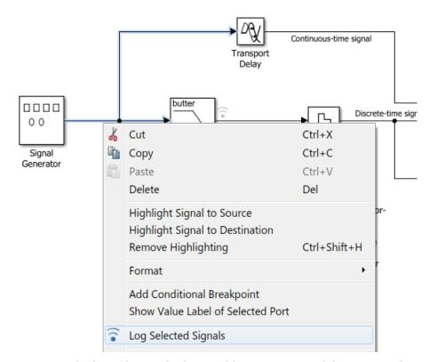
• Use any method to select multiple signal lines in your model. For example, use **Shift**+click to select multiple lines individually or **CTRL+A** to select all lines at once. Then, on the **Signal** tab, select the **Log Signals** button.
