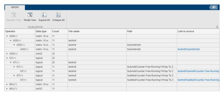
The result shows that the ADD operator is used 11 times with data type matrix 10 uint32, and 22 times with data type uint32. The GT (greater than) operator was used 22 times total with data type logical: 11 times from **SubAdd** model, and 11 times from **SubMult** model. The MUL operator is used 11 times with data type uint32, and 11 times with matrix 10 uint32.
