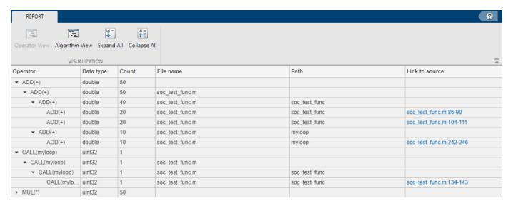
The result shows that the ADD operator is used 50 times with data type double. The call to myloop executes once with data type uint32, and the MUL operator is used 50 times with data type uint32.
