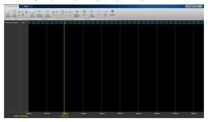
1 In the **Logic Analyzer**, click the arrow next to a fixed-point or integer wave to view the bits.
